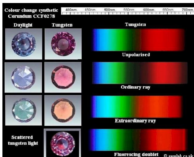
Fig. 21.: Synthetic corundum laced with vanadium have refractive index of 1.759 - 1.776 , contains gas bubbles and shows a characteristic
